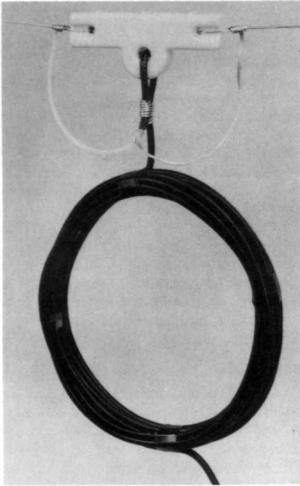
Fig 3—A coaxial-cable choke balun with an air core is effective and light enough to hang from the feed point of a well-supported dipole antenna.
